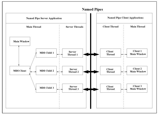
Figure 163. Named Pipe Sample Program Architecture
